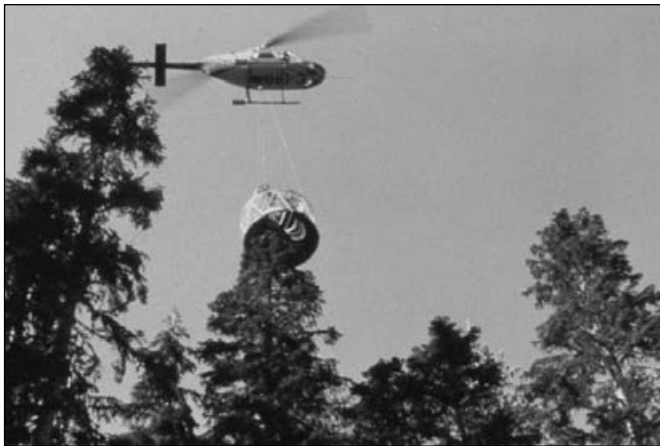
Figure 13 — Abies procera , noble fir: aerial collection using a cone rake (courtesy of D. Pigott).
