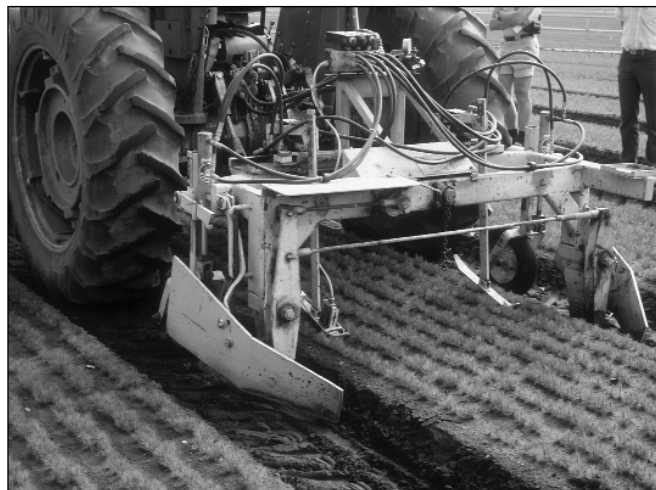
Figure 13 —Chapter 7, Nursery Practices: root culturing is important to develop a fibrous root system. These pine seedlings are being wrenched with a sharp-angled blade that is being pulled under the seedbed.
