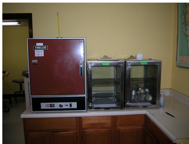
Figure 9 —Chapter 5, Seed Testing: a convection oven and desiccator are used to conduct a seed moisture test.
