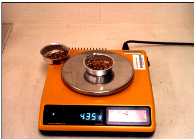
Figure 8 —Chapter 5, Seed Testing: 2 seed samples are tested to measure the moisture content of a seedlot.
