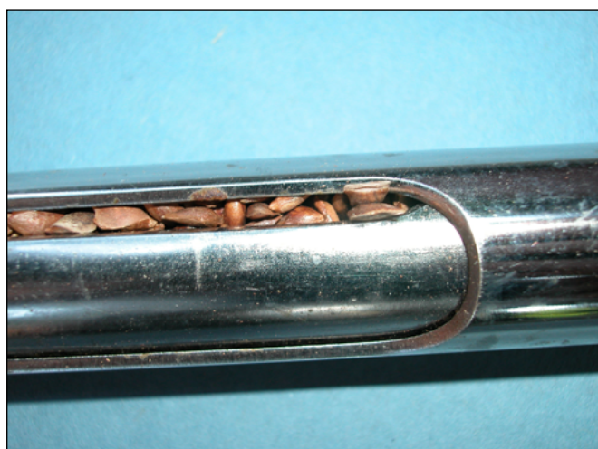
Figure 2 —Chapter 5, Seed Testing: seeds caught in the gates of the seed probe must not be cut when the gates are closed.
