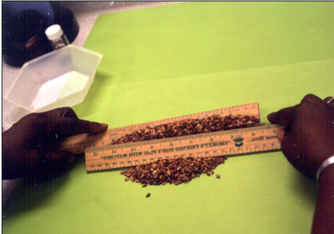
Figure 6 —Chapter 5, Seed Testing: the composite sample is divided systematically into quarters, eighths, sixteenths, and smaller fractions to obtain the submitted sample at the seed storage plant or the working sample in the laboratory.
