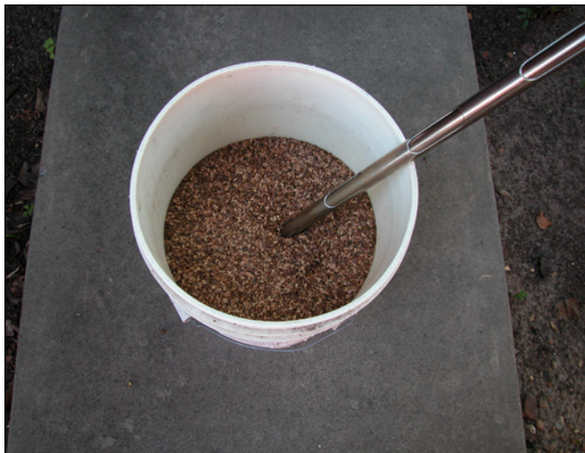
Figure 1 —Chapter 5, Seed Testing: seed probes are used to sample free-flowing seeds.
