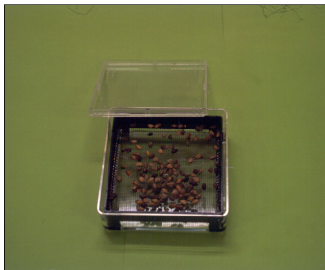
Figure 24 —Chapter 5, Seed Testing: the accelerated aging test is conducted by placing seeds in a plastic box with a water reservoir and holding them at 40 °C for 72 hours.
