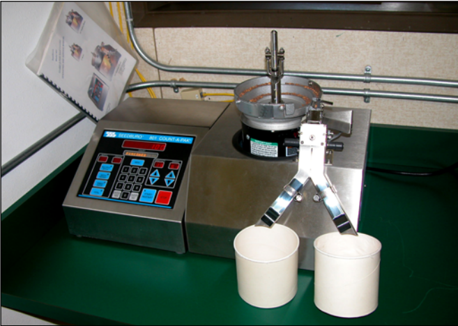
Figure 18 —Chapter 5, Seed Testing: an electronic seed counter is sometimes used to estimate the number of seeds per weight (in either kilograms or pounds).
