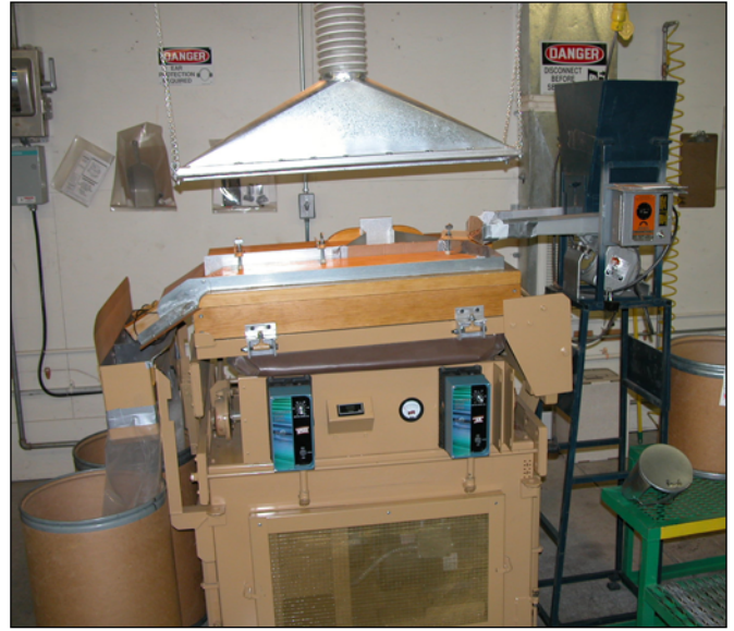
Figure 37 —Chapter 3, Seed Harvesting and Conditioning: a specific gravity table for separating seeds and trash by weight.
