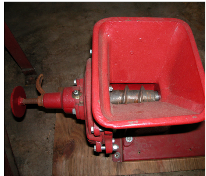
Figure 16 —Chapter 3, Seed Harvesting and Conditioning: a grinder can also be used to crush fleshy fruits for seed extraction.
