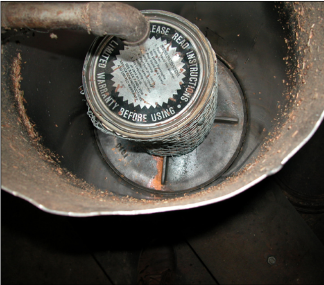
Figure 14 —Chapter 3, Seed Harvesting and Conditioning: maceration time is reduced by adding to the macerator a hardware cloth liner and a can wrapped with hardware cloth.
