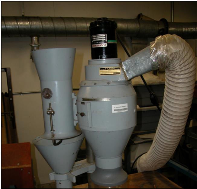
Figure 26 —Chapter 3, Seed Harvesting and Conditioning: a laboratory aspirator removes trash with vacuum.
