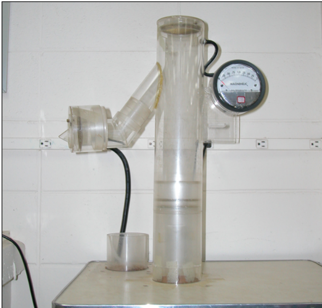
Figure 27 —Chapter 3, Seed Harvesting and Conditioning: a laboratory blower removes trash with positive pressure.
