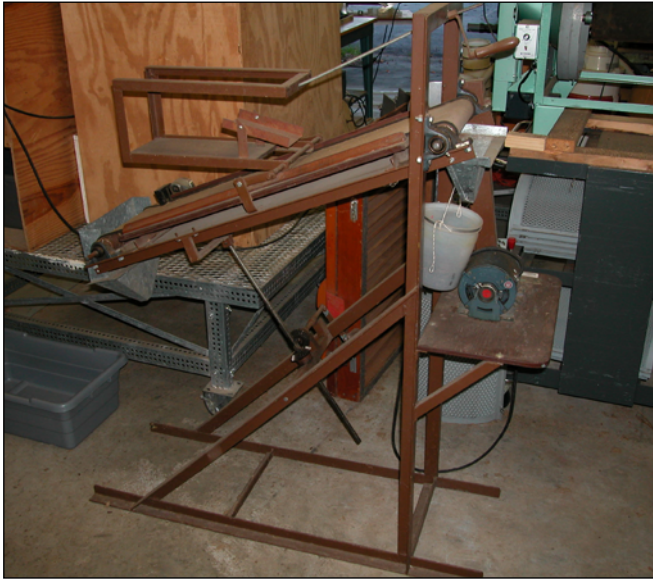
Figure 36 —Chapter 3, Seed Harvesting and Conditioning: the inclined draper separates particles on their ability to roll or slide down the inclined belt.
