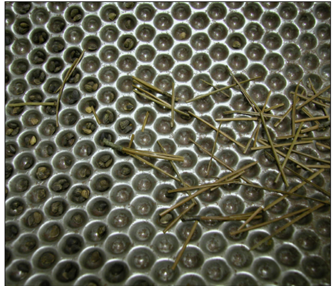
Figure 32 —Chapter 3, Seed Harvesting and Conditioning: seeds are caught in indent cylinder while pine needles slide away
