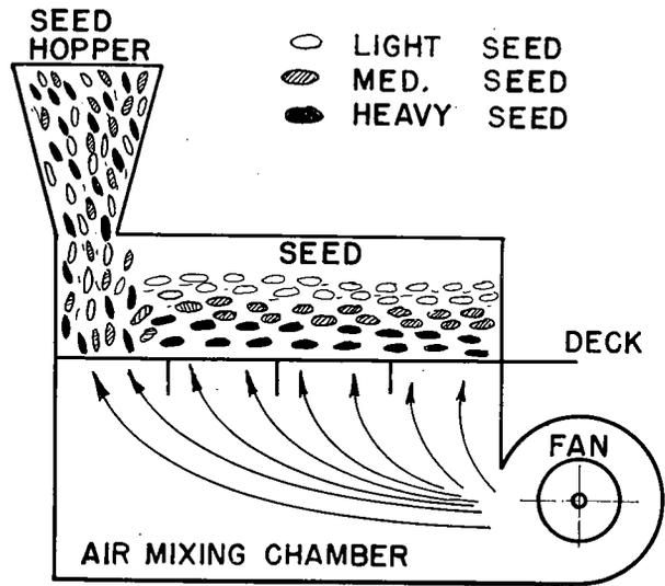
FIGURE 11.—Cross section of specific gravity separator.
