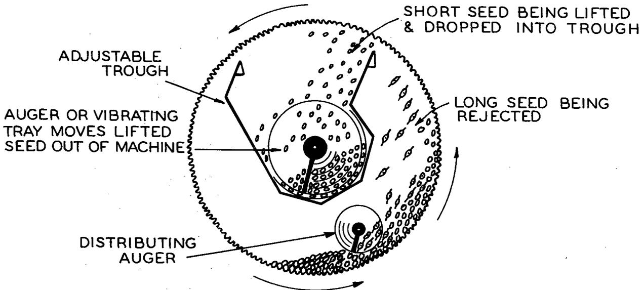
FIGURE 8.—Cross section of an indent cylinder separator.
