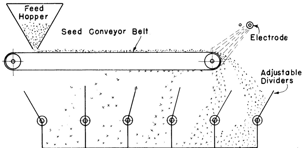
FIGURE 27.—Schematic drawing of an electrostatic seed separator.
