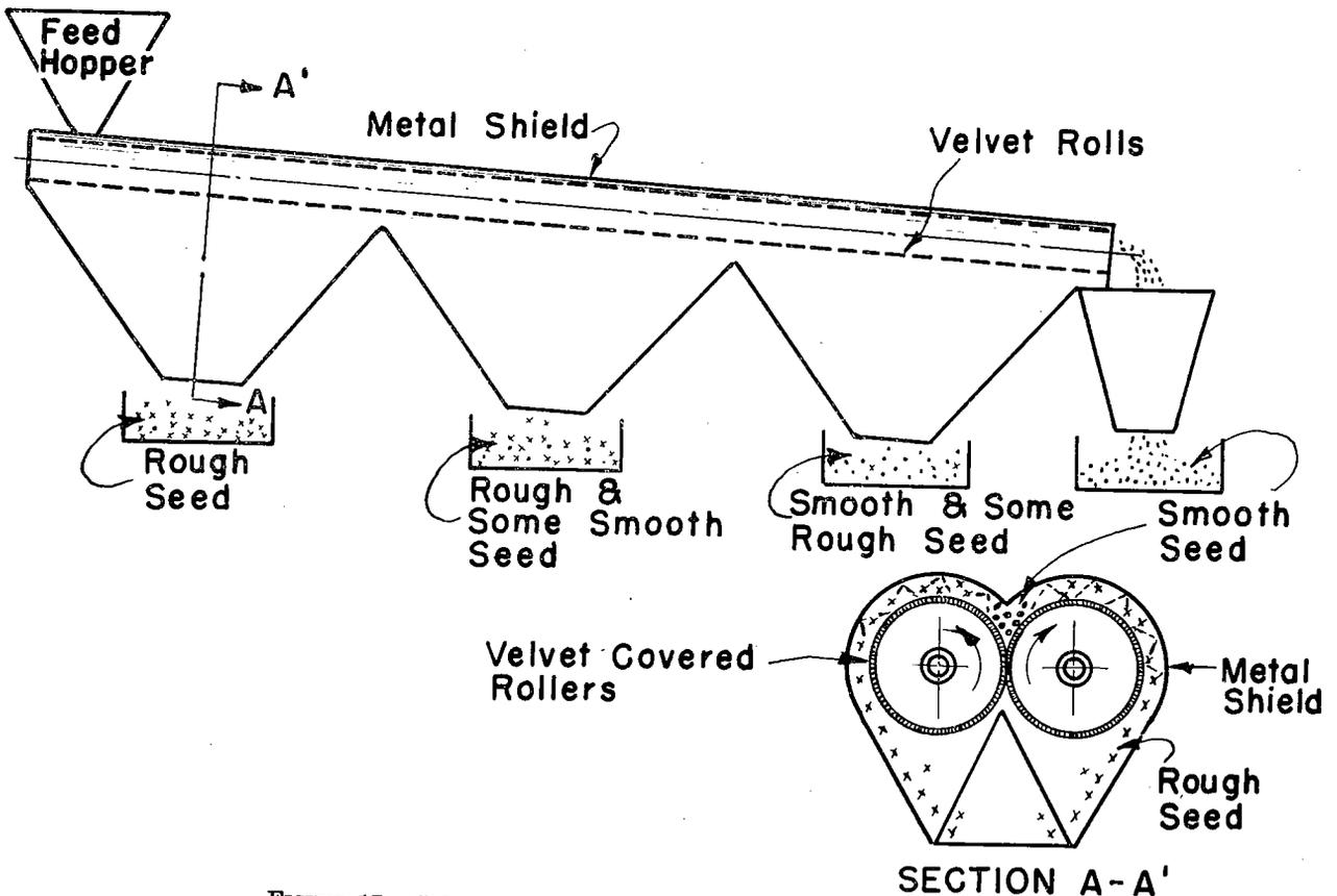
FIGURE 17.—Side view and cross section of velvet roll separator.
