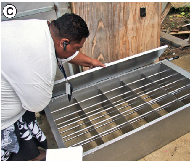
Figure 6.11 —For nurseries making their own media, pasteurization with steam (A) or wood heat (B) is simple, effective, and can be accomplished with portable equipment. Electric soil sterilizers can heat the soil long enough to eliminate most weed seeds and pathogens (C). Photos A and B by Thomas D. Landis, and photo C by J.B. Friday.
