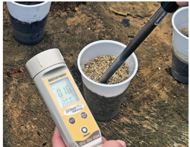
Figure 6.16—Growing media salinity can be measured using an EC meter. Photo by J.B. Friday.
