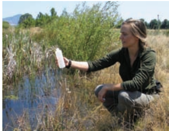
Figure 10.4 —Water quality should be tested before nursery establishment, and then yearly to make certain that quality has not changed. Photo by Thomas D. Landis.
