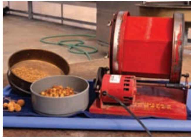
Figure 8.6 —Hobby-size rock tumblers can be used to scarify seeds. This method is an effective alternative to acid or heat scarification. Photo by Tara Luna.
