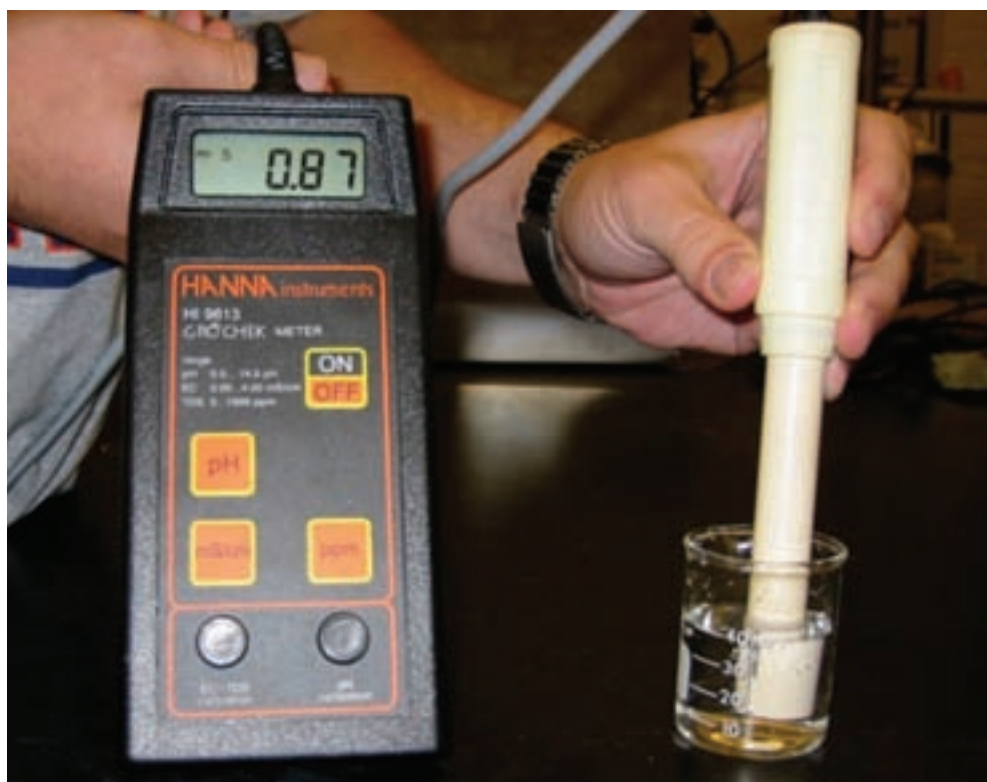
Figure 11.12 —An electrical conductivity meter used to estimate fertilizer salt concentrations in irrigation water, fertigation water, or saturated media extract. Photo by Douglass F. Jacobs.
