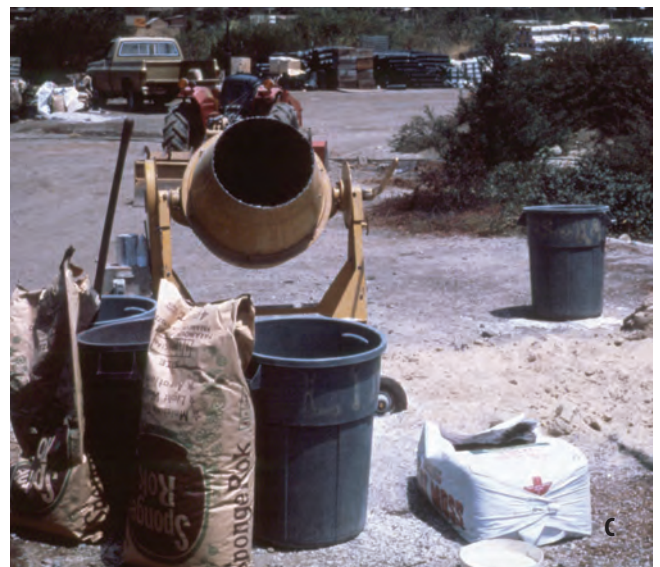
Figure 5.10 —(A) Nurseries that mix their own media should first screen materials and then (B) mix them thoroughly using the moving pile technique. (C) To reduce labor, a cement mixer can also be used but care must be taken to avoid overmixing and the resultant damage to particle size and structure. Photos A and B by Thomas D. Landis, C by Tara Luna.
