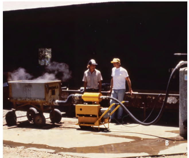
Figure 5.12 —(A) Some commercial growing media have been pasteurized to kill pathogens. (B) For nurseries making their own media, pasteurization with steam or solar heat is simple, effective, and done with portable equipment. Photos by Thomas D. Landis.
