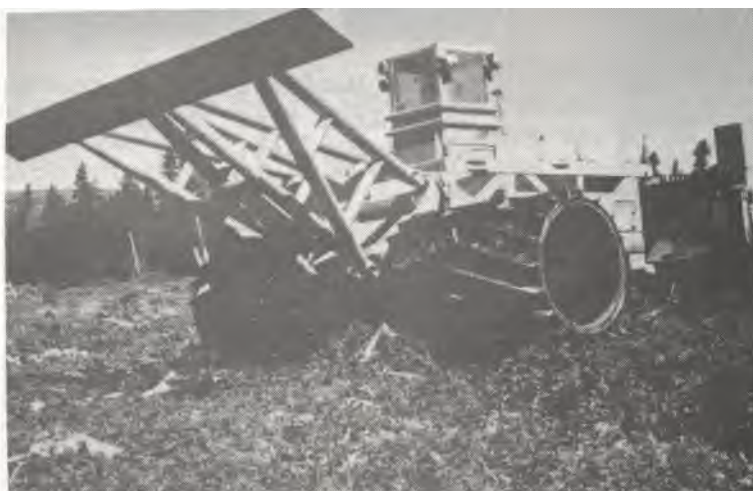
Fifty-ton crusher. Bar is for pushing over residual trees and drum-type wheels crush woody material on ground.
