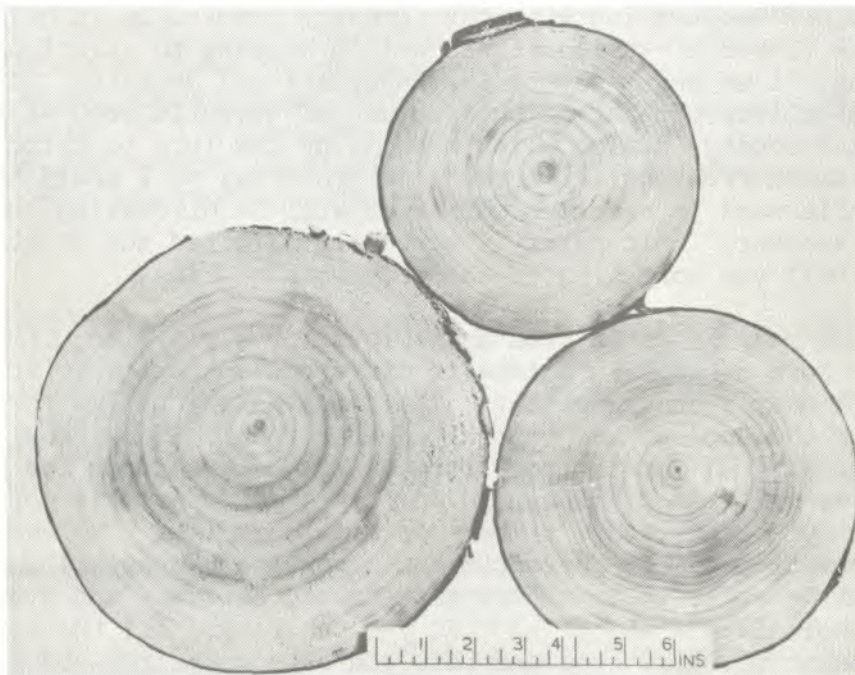
Figure 2.-- Picea sitchensis, 28 years old. Cross sectional disks at 20 ft. and 40 ft. levels, showing large proportion of juvenile wood
