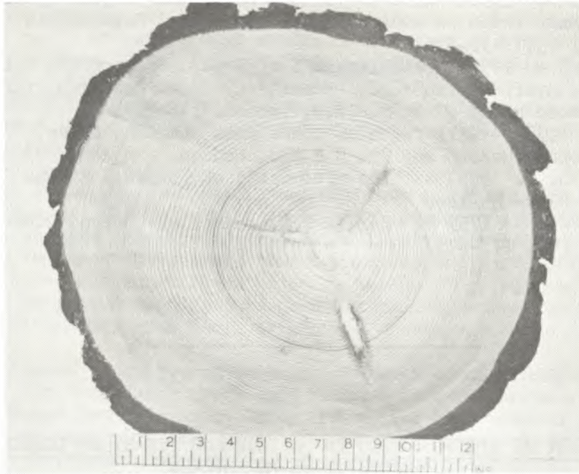
Figure 1.-- Cross sectional disk of Pinus sylvestris, 89 years old, showing small proportion of juvenile wood
