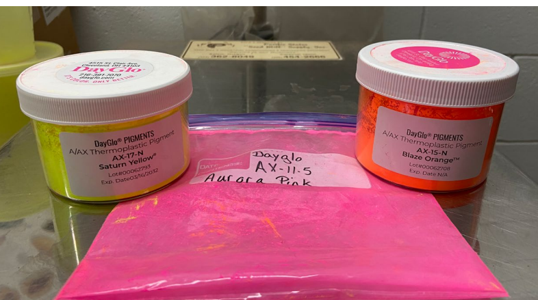
Figure 2. DayGlo manufactures a range of daylight fluorescent pigments. As per the company website, the “A and AX series pigments are thermoplastic, fluorescent pigments recommended for a wide range of applications where resistance to strong solvents is not needed, including paper coatings, vinyl coated fabric, A-type gravure inks, paints, screen inks, and vinyl plastisols and organosols” (DayGlo Color Corp. [N.d.]). Photo by Jacob Witcraft, 2024.
