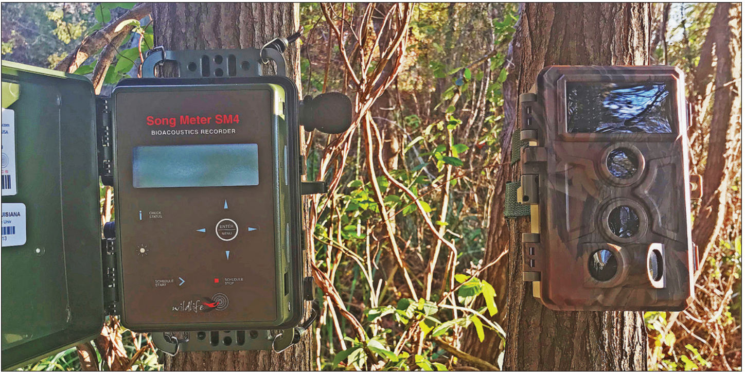
Figure 8. The SM4 song meter (left) and a motion-activated trail camera (right) were used to document avian herbivory in Trial Two. (Photo by Heidi Adams, 2021).
