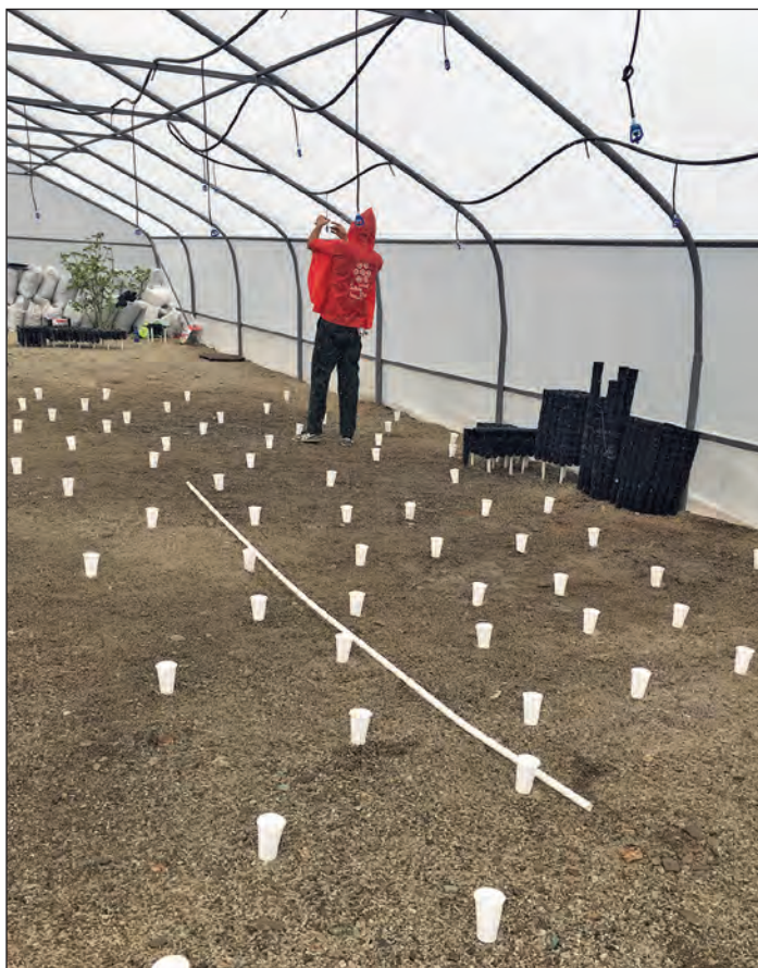
Figure 1. A cup test measures the amount of irrigation water that fills cups in a set amount of time. This test is used to determine the application rate of the irrigation system and accounts for the cumulative flow rate of multiple sprinkler heads across the growing area. (Photo by Rebecca Sheridan 2017)
