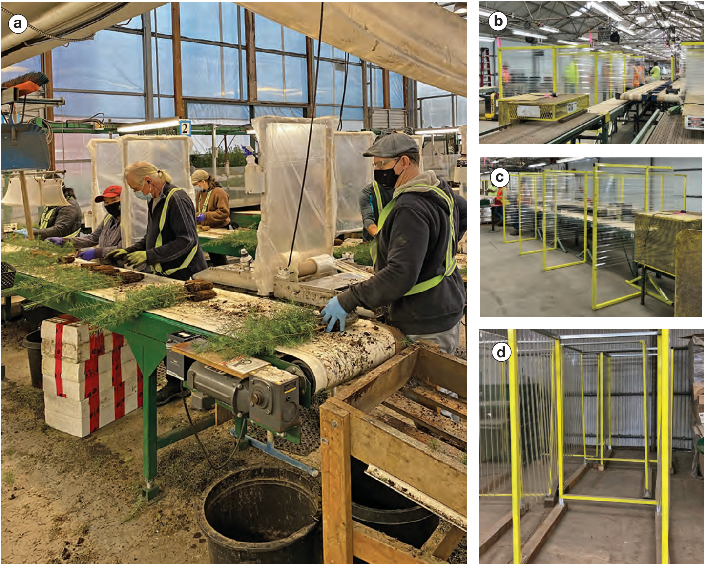
Figure 4. Some nurseries have constructed barriers as part of conveyor lines to separate workers from one another. Individual sanitation bottles are often provided at each station for frequent sanitation. (Photos by Thomas Stevens and Sean Webb 2020)
