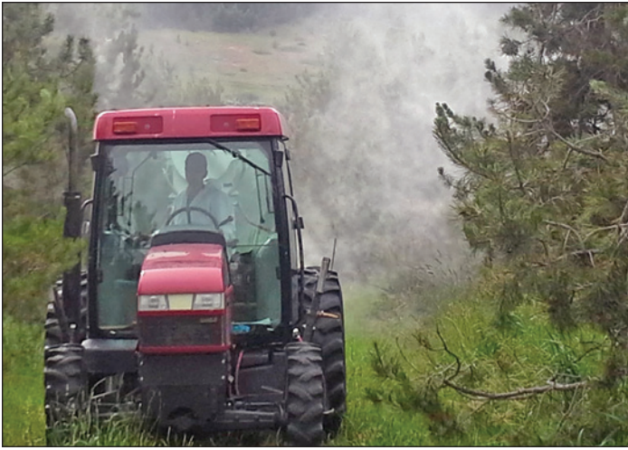
Figure 11. For trials 3 and 4, insecticide treatments were applied with a commercial air blast sprayer. This is the standard application equipment in commercial forest seed orchards. (Photo by Mario Lanthier 2017)
