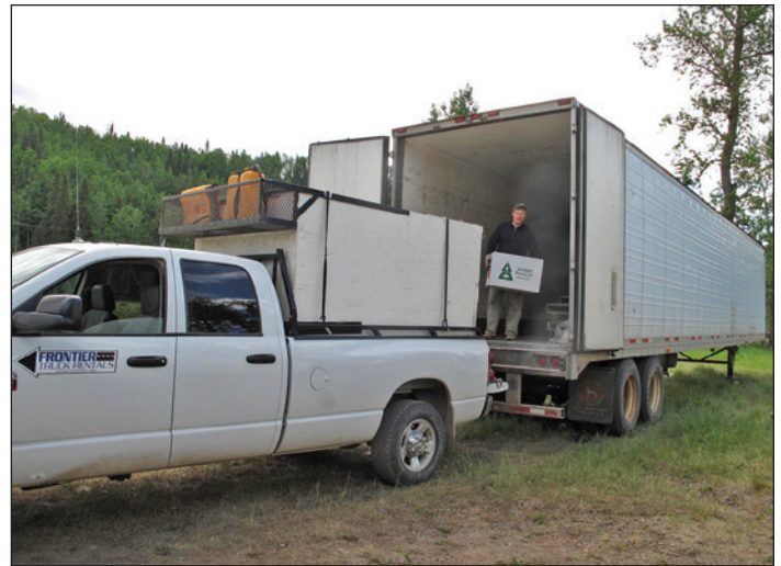
Figure 5. Refrigerated trailers are required for transporting large quantities of hot-lift seedlings from the nursery and are ideal for short-term cool seedling storage prior to planting. (Photo by Steven B. Kiiskila 2010)
