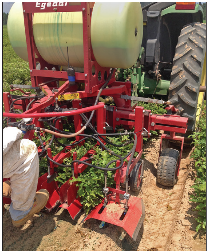
Figure 2. At some nurseries, liquid ammonium polyphosphate is applied to hardwood seedbeds in May, June, July, and August using directed sprayers. The shield reduces the amount of fertilizer applied to the tire-paths and increases the amount of phosphorus applied to the soil. (Photo by Robert Cross 2014).
