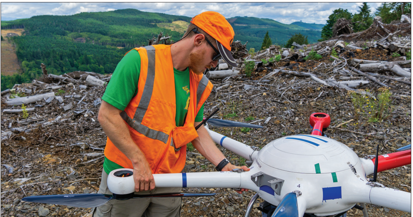
Figure 1. A DroneSeed custom-engineered hexacopter (patent pending) capable of carrying up to 57 lb (25 kg) of payload with an “all-up” weight up to 115 lb (52 kg). This aircraft is typically flown autonomously as part of multiple, coordinated, high-capacity, autonomous aircraft, also known as “swarms,” and operated by a limited number of ground personnel to service battery and payload replacements between missions. (Photo courtesy of DroneSeed 2019)
