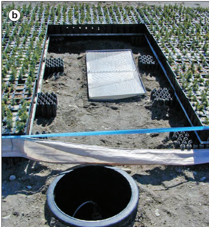
Figure 2. (a) Large 2+0 white spruce grown outdoors in 25-310 containers at the Saint-Modeste nursery were fertilized and irrigated with a mobile boom. (b) Stainless steel leachate collector and its recovery well for measuring leaching losses under containerized 2+0 white spruce seedlings at the Saint-Modeste nursery. (Photos by Daniel Girard, 2009 and 2003)
