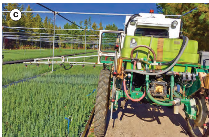
Figure 1. (a) Large 2+0 white spruce grown outdoors in 25-350A containers at the Normandin nursery with weather station position above the containers to monitor environmental variables. (b) Leachate collector used to measure the losses of substrate solution under seedlings. (c) Tractor-mounted boom sprayer used to fertilize 2+0 container seedlings at the Normandin nursery. (Photo (a) by Daniel Girard, 2000; Photo (b) by Daniel Girard, 1999; and photo (c) by Jean Gagnon, 2016)
