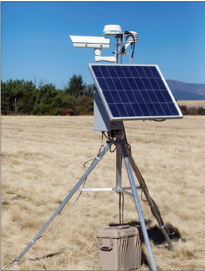
Figure 1. Remote monitoring system with tripod-mounted camera, solar panel, and battery. (USDA Forest Service photo)
