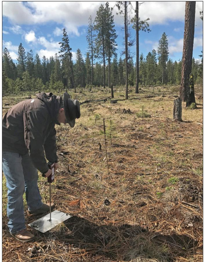
**Figure 3.** Soil density was measured on both units using a soil densiometer. (Photo by Jack Rigglin, 2017)
