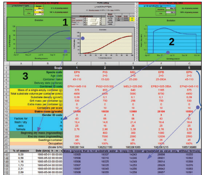
Figure 11. For each scale, the mass that is not substrate water is predicted by simulation for each day of the upcoming growing season. (1) A general profile is set for the seasonal evolution of dry mass, from 0 to 100 percent of the final value, using tools in the grey section. Thereafter, the beginning and the end of the growing season are established to fix the x-axis for the nursery. (2) To obtain the fresh mass, a standard “fresh/dry” ratio of 3.5 can be used, but up to five seasonal evolution profiles of fresh/dry ratios can be established according to the genus of seedling crop ( Picea : EPN, Pinus : PIG, Larix : MEL, etc.) to give more precise results. (3) The profile of the dry mass is adjusted according to the targeted dry mass values for the crop of each scale (y-axis). All other parameters (grey zone, red characters) are taken into account to calculate the mass that is not substrate water for every scale and for each day of the growing season (purple zone). Note that all values shown in the third section are given by spreadsheet formulas. In the next step (figure 12), these data will be used to easily produce and show the volumetric water content of the substrate.
