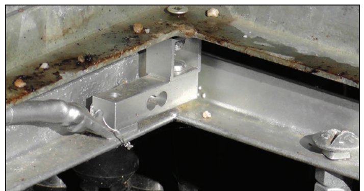
Figure 6. One of the four low-cost load cells used for a scale (bending beam type, protected by a simple coat of aluminum-based paint) after a growing season in the forest nursery. A 3.2 mm (0.125 in) spacer is needed between the lower bed and the load cell, and a 19 mm (0.75 in) spacer is required between the other side of the load cell and the upper bed to mechanically insulate the beam from any unwanted contact. Mass applied on the upper bed induces invisible deformations on the beam that are perceptible by strain gauges applied on it. The initial result is a variable electrical signal (voltage) that is linearly related to the containers' mass. (Photo by Daniel Girard, 2014)
