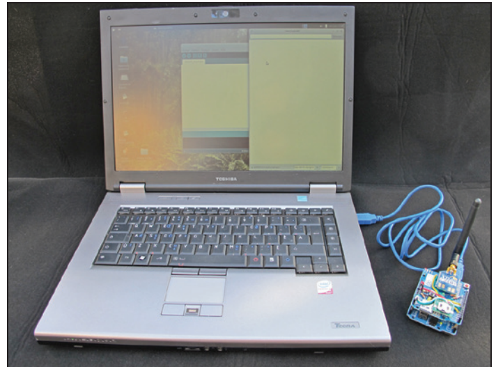
Figure 4. Receiver (stand-alone datalogger) connected to a computer to show in real time the incoming weighing data. (Photo by Daniel Girard, 2016)
