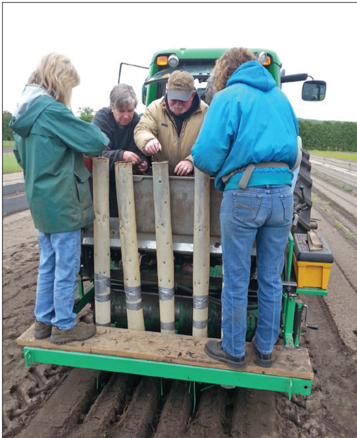
Figure 4. The nursery's Whitfield hardwood tree planter was modified with drop tubes to hand-feed bundles of aspen roots for planting. (Photo by Joseph Vande Hey, 2015)
