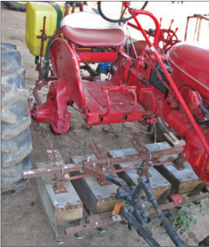
Figure 6. This photograph shows an example of a shielded herbicide applicator designed for hardwood seedbeds. The advantage of this model is that one person can operate it. (Photo by David South, 2010)
