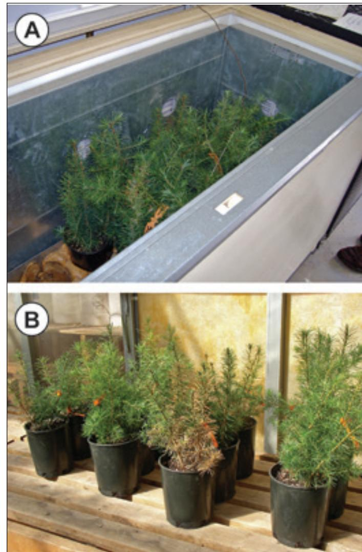
**Figure 2.** (a) A programmable freezer was used to subject seedlings to the whole plant freeze test. After freezing, seedlings were kept in (b) ambient conditions before assessing for freeze damage. (Photos by Diane L. Haase, 2006)
