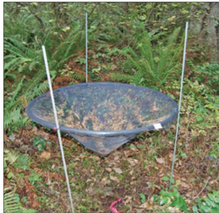
**Figure 1.** Each seedtrap contained a circular frame, 1.0 m<sup>2</sup> (10.8 ft<sup>2</sup>) in area, constructed of flexible plastic tubing. A semicircle of fiberglass screen was stapled to the frame to create a conical trap for collecting Douglas-fir seeds, cones, and other forest litter. The trap was suspended on rods approximately 0.75 m (2.5 ft) above the ground. (Photo by Timothy B. Harrington, 2008)
