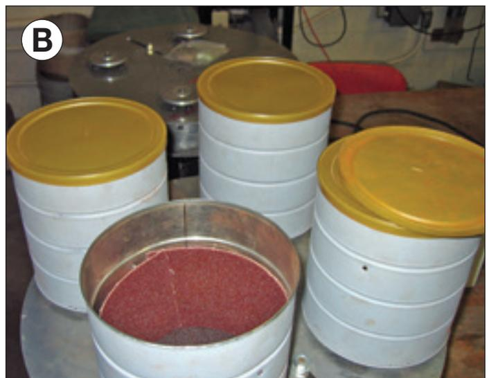
**Figure 2.** The USDA Forest Service, Missoula Technology and Development Center developed this rotary drum sander to scarify seed (Gasvota et al. 2002). (a) Seed is placed in each coffee can lined with 50-grit sandpaper and (b) seeds are scarified for 3 hours at 70 revolutions per minute. (Photos by Nathan Robertson and Emily Overton)
