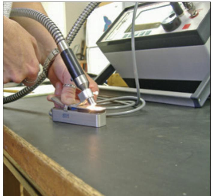
**Figure 4.** After freezing, chlorophyll fluorescence was measured on needles from Nursery A by exposing needles to a pulse of saturating light using a fluorometer. (Photo by Diane L. Haase, 2006)
