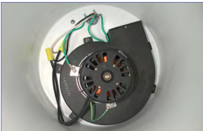
Figure 5. Placement of the induced draft blower and wiring in the bottom of the 5-gal (19-L) bucket. (Photo by Robert Karrfalt)
