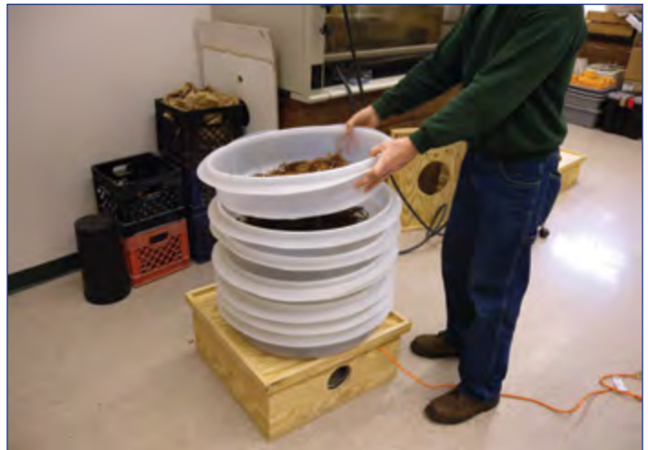
Figure 7. Pressurized dryer made with 55-gal (208-L) barrel paint strainers. (Photo by Robert Karrfalt)
