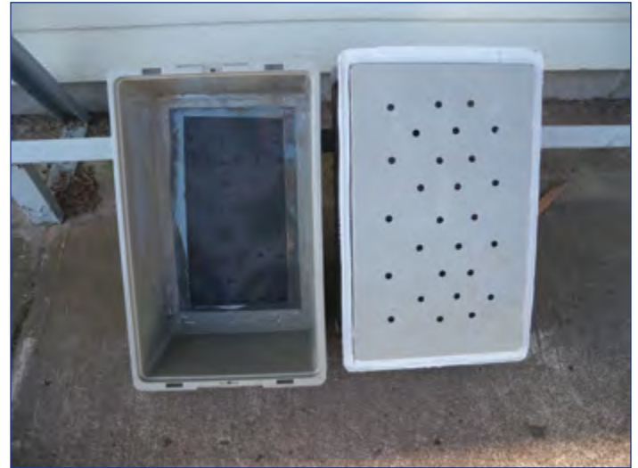
Figure 10. Box on the left shows pet screen taped to the bottom and box on the right shows hole pattern and foam gasket. (Photo by Robert Karrfalt)
