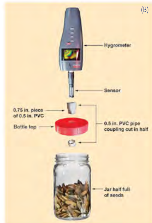
Figure 3. (A) Hygrometer inserted into closed jar to measure the equilibrium relative humidity of a seed sample. (B) Schematic representation of the hygrometer, insertion port, and sample jar. (Photo by Robert Karrfalt and illustration by Jim Marin)
