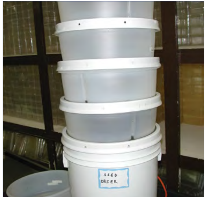
Figure 4. Pressurized seed dryer made from a 5-gal (19-L) bucket, paint strainers, a furnace motor, and other readily available parts. (Photo by Robert Karrfalt)
