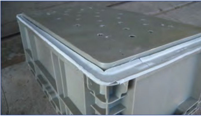
Figure 11. A foam gasket is needed on the flange on the bottom of the drying box to form an airtight seal. (Photo by Robert Karrfalt)
