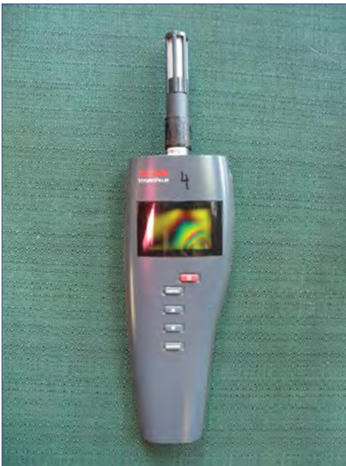
Figure 2. Hand-held hygrometer for measuring relative humidity in drying area and equilibrium relative humidity of seed samples. (Photo by Robert Karrfalt)
