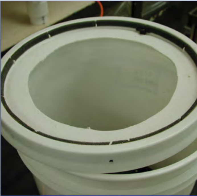
Figure 8. The lid of the 5-gal (19-L) bucket should have the center removed, leaving a 2- to 3-in (5- to 7-cm) lip. In addition, attaching 0.25-in (0.6-cm) thick foam insulation will improve the seal between the lid and the paint tray that will sit upon it. (Photo by Robert Karrfalt)
