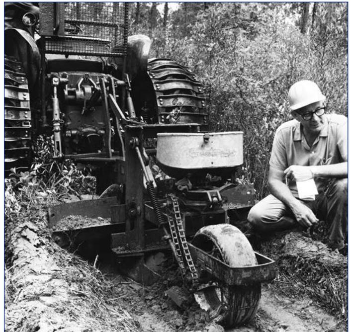
**Figure 11.** Thomas C. Croker demonstrating a row seeder that elevates a low ridge in a plowed furrow and drops seeds that will be pressed into the soil. (Photo from USDA Forest Service files circa 1962)
