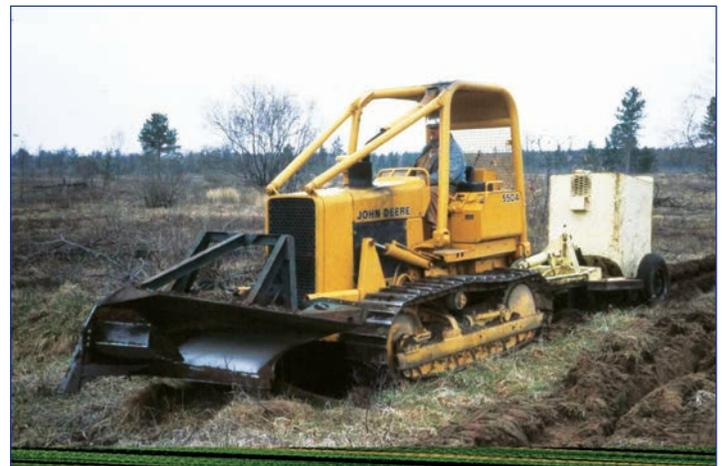
Figure 5. Whitfield planting machines (left and right) mounted on John Deere bulldozers were used for several years, circa 1980. (Photos from MDNR files)
