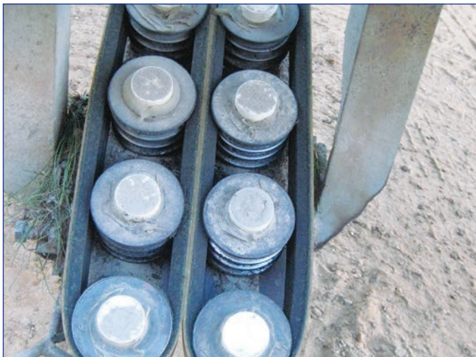
Figure 4. One row of lifter belts for the Mathis® two-row lifter. (Photo by Tom E. Starkey)
