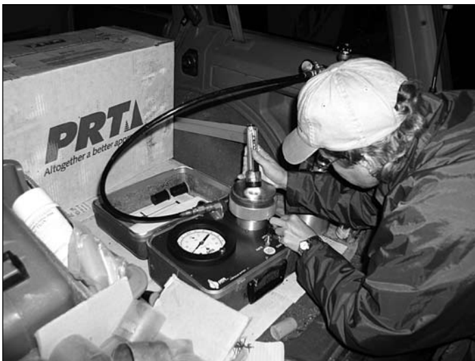
Figure 8. A pressure chamber is used to determine the xylem water potential of a seedling branch sample.
