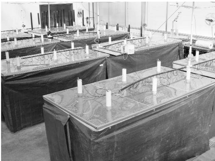
**Figure 1.** Operational rhizotrons used for two-dimensional, horizontal root growth measurements. Observations of the root systems are taken on the underside of the rhizotrons by removing the tarps.
