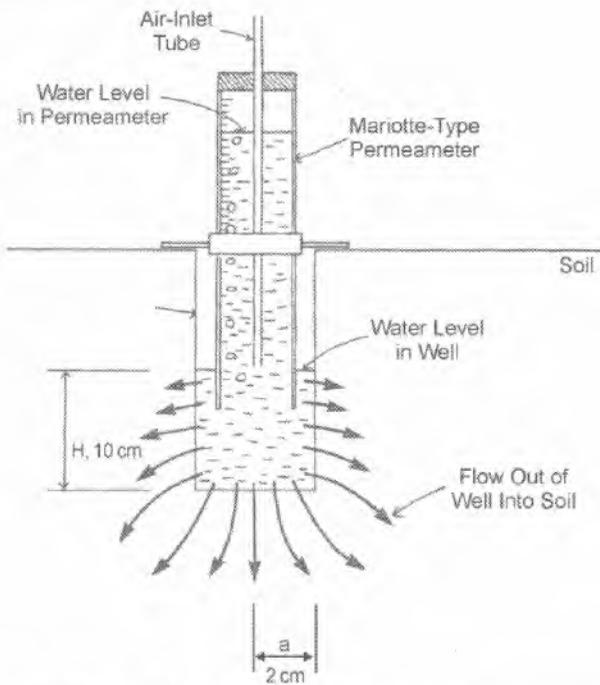
Figure 1. The head of the in-hole Mariotte-type permeameter.
