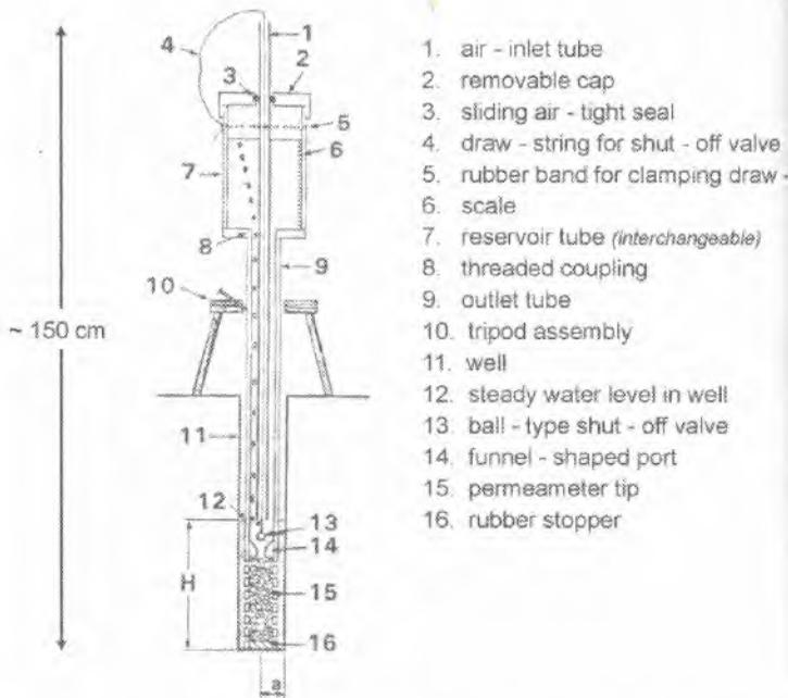
Figure 2. The constant-head well permeameter in position.
