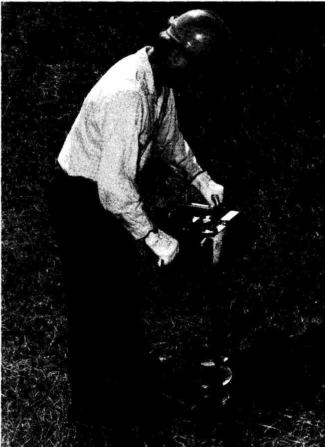
Figure 1 —Power-driven auger that produces a cone-shaped hole.
