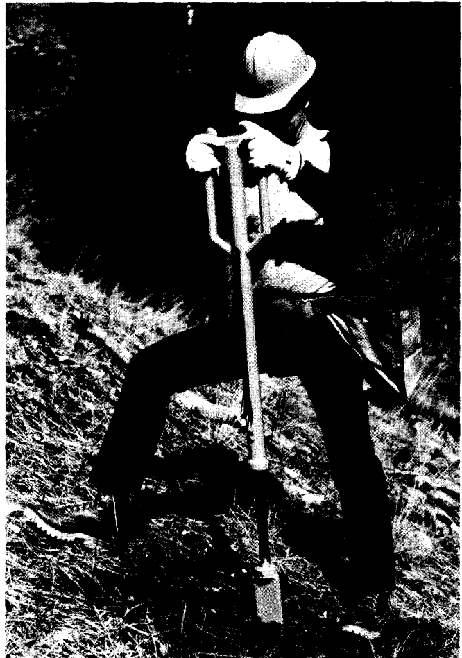
Figure 2 —Hammer-action hand planter with a double-D handle.
