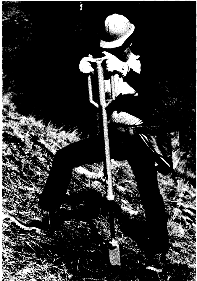
Figure 2 —Hammer-action hand planter with a double-D handle.
