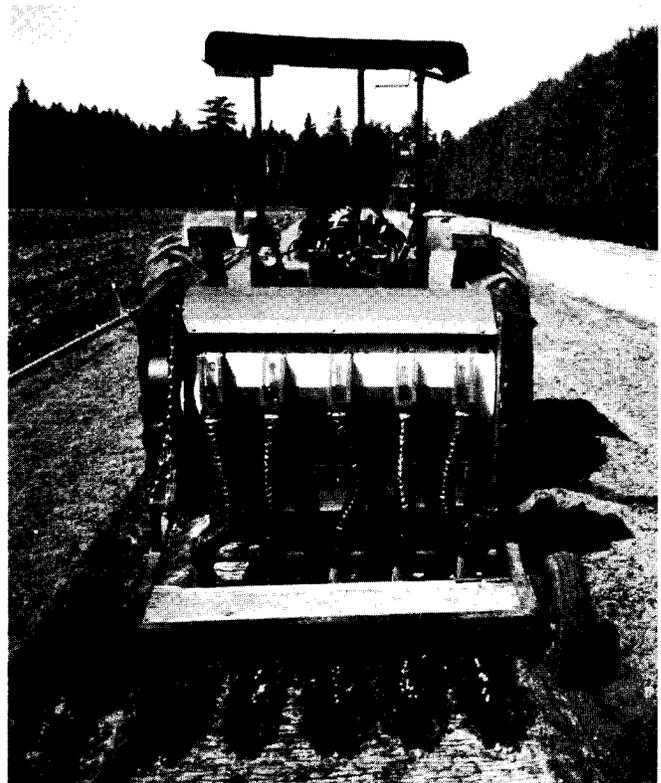
Figure 1—Ground-driven seeder sowing 5 rows of acorns.
