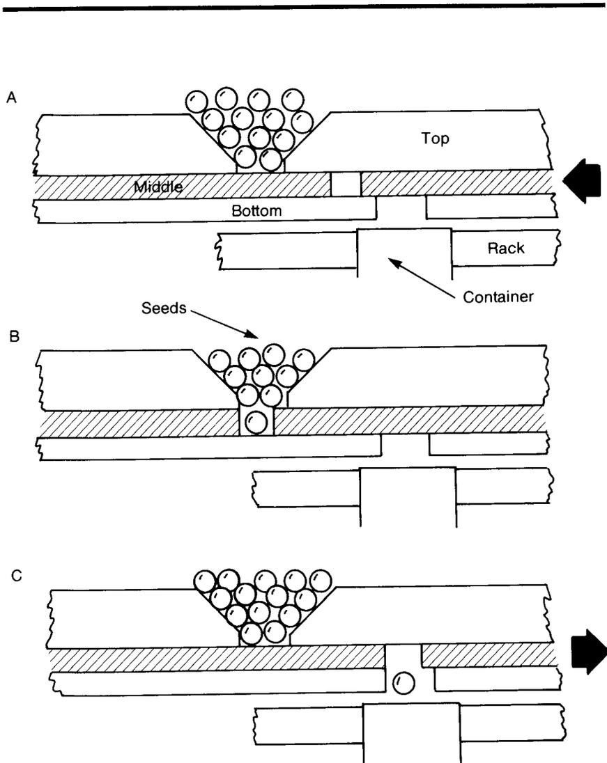
seeder, moving the middle plate back and forth (sowing the seeds), and removing the containers requires about 15 seconds. If more than one seed is required in each container, the middle plate is moved back and forth as many times as needed to sow the correct number of seed.
