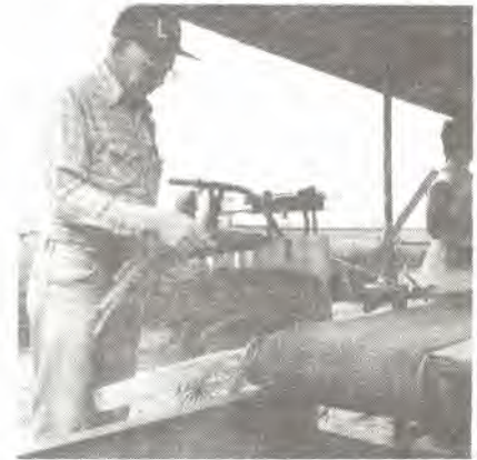
Figure 7—A taping machine secures the Tinus Roottrainers in units of 32 seedlings.
