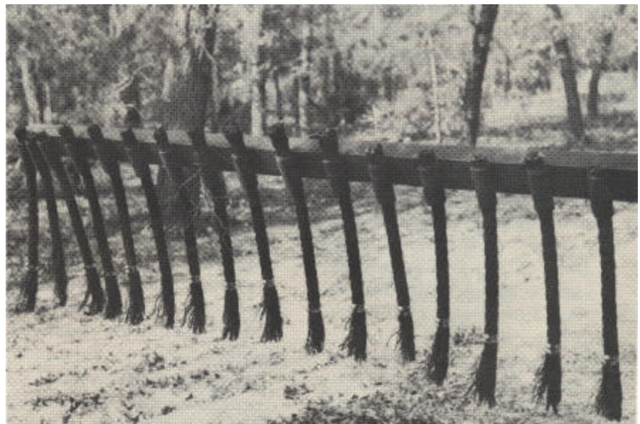
Figure 2. —Steel cable segments on scarifier.
