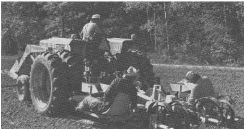
Figure 3.—The tree-planting interval indicator in use with semimanual transplanters at the experimental farm of the forestry Sciences Laboratory, Rhinelander, Wis.
