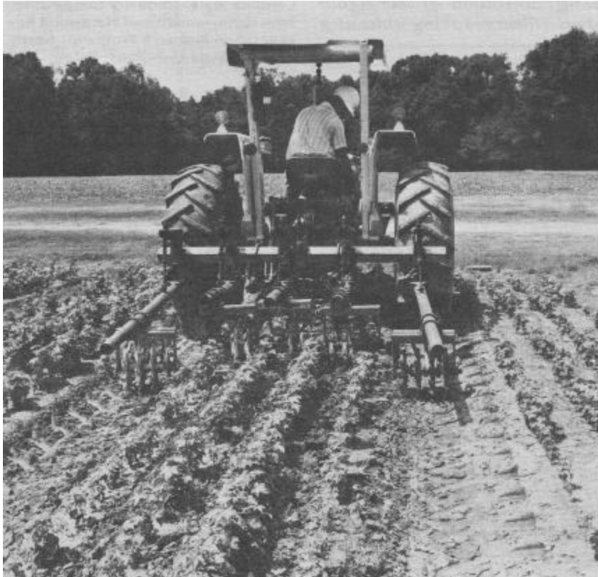
Figure 1. —Modified Lilliston rolling cultivator with five adjustable modules cultivating 8-week-old sweetgum in nursery seedbeds.
