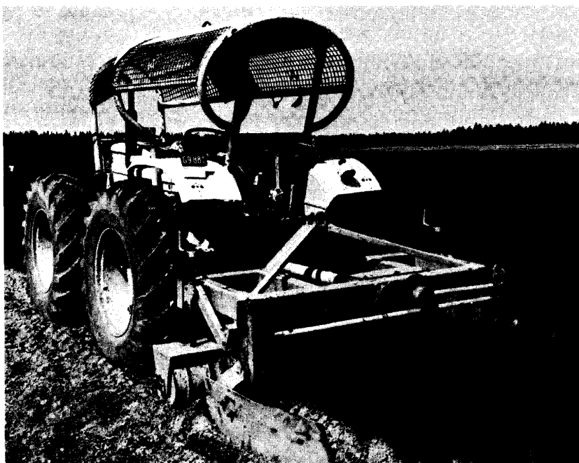
Figure 2. —Reciprocating root wrencher used for conditioning 1-0 pine planting stock in Queensland.
