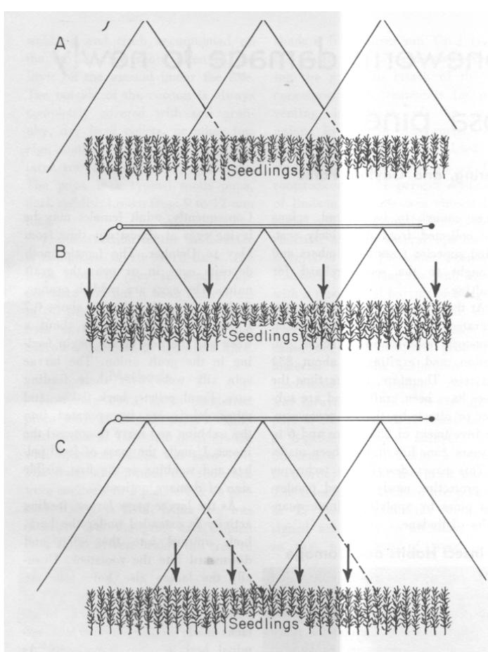
Figure 3.-Side view shows proper and improper spray patterns: (A) proper height of spray nozzles results in uniform water distribution; (B) nozzles too close to seedlings result in too little water in spray overlap areas and at edges; (C) nozzles too far above seedlings result in too much water in the spray overlap area and at edges. Arrows show areas where water distribution is not uniform.
