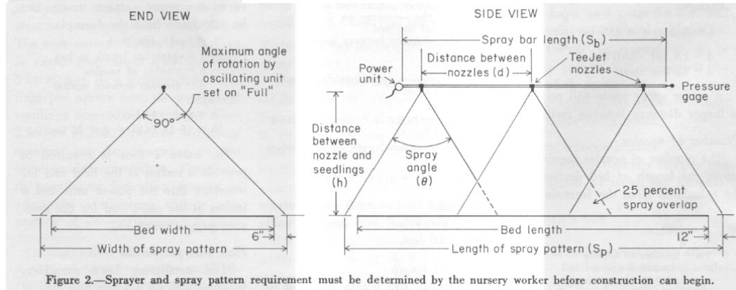
Figure 2.—Sprayer and spray pattern requirement must be determined by the nursery worker before construction can begin.
