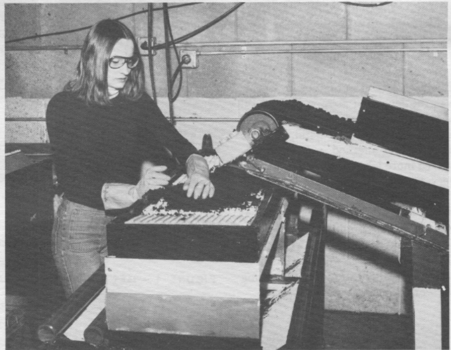
Figure 4.—Once peat is mixed in batch mixer, it drops onto conveyor which elevates to shaker table. Here, the moist peat is spread over the containers. As the peat is shaken down, more is added to completely fill container.
