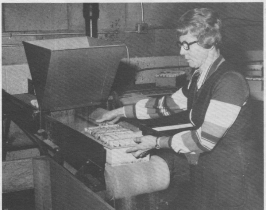
Figure 6.—Gritting with clean, dry sand. Hopper is filled periodically. Excess sand falls into tub to be recycled after cleaning on sieve table. This operation fills 55,000 cavities per day.
