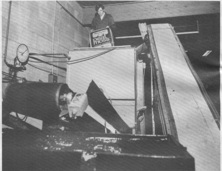
Figure 3.—Filling the batch mixer is first step in process. Peat is mixed to 85 percent water capacity. Meter (left center) controls water input for mixing.
