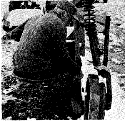
Figure 2.—Rear view of planter showing width of trencher; also the position, size, and shape of the packer wheel.
