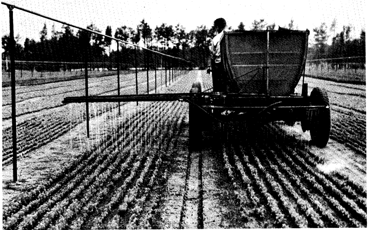
Figure 3.—Multiuse sprayer with a pressure pump and agitators that apply rapidly liquid fertilizers, acidifying solutions, and hydrosolic eradicans.
