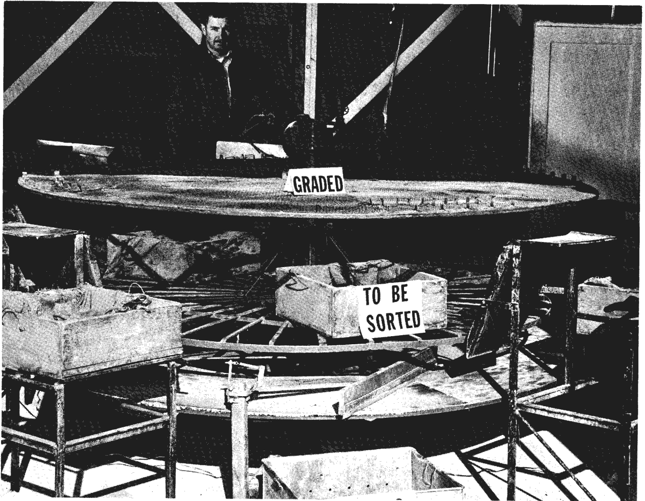
Figure 1.—Three-level sorting wheel: Top level for graded trees; middle level for boxes of trees; lower level for culls.
