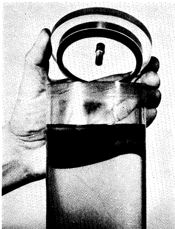
Figure 1.—The slide-in cap fitted with an O-ring and tire valve provides a tight seal and eliminates air compression and displacement error encountered with the screw cap.
