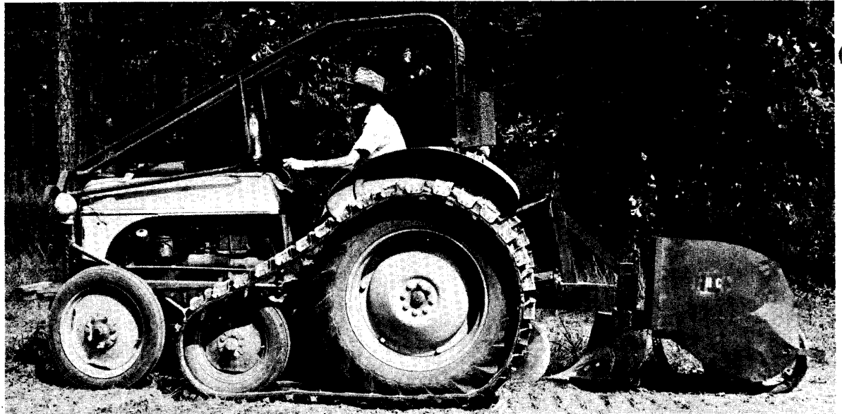
Figure 2.—In the compact H-C seeder, the scalper, bedder, sower, and packer are all in one compact unit which can be attached to any tractor with a standard three-point hitch. It is good for small open areas.
