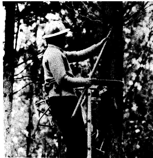
Figure 1.--Overall view of the Morris high-pruning equipment. (Courtesy of New Zealand Forest Service.)
