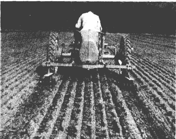
Seedbed cultivator blades break up crust of soil between rows of seedlings; two sets of disks cultivate paths.
