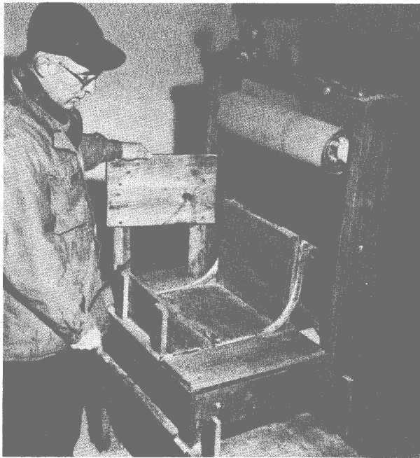
Figure 1--Packing table: Left, Steel tape being fed into aluminum channel guide; right, steel tape being brought from tape reel into position for bundling.
