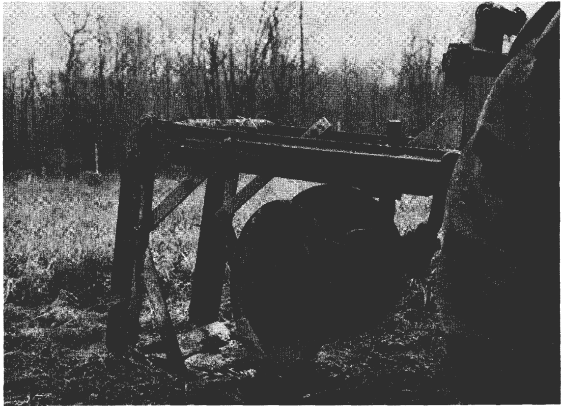
Figure 1. - Lifter in action. Chain hook up and turnbuckle determine angle of blade at a certain depth. The 1-inch bolt holding blade to hanger has a double nut to allow blade to swing.
